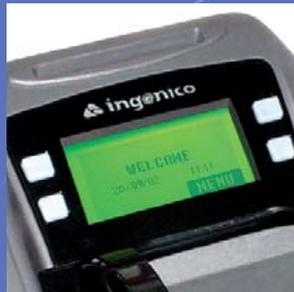
4 soft keys simplifying application selection
